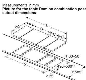
If two or more elements are installed right next to one another, one or several installation kits are required (2 elements 1 installation kit, 3 elements 2 installation kits, etc.)
