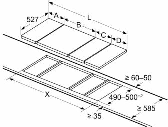
If two or more elements are installed right next to one another, one or several installation kits are required (2 elements 1 installation kit, 3 elements 2 installation kits, etc.)
